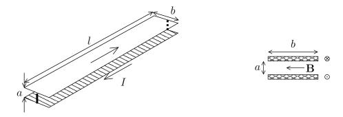
Assume that the magnetic field strength  $\mathbf{B}$  is constant between the plates when a steady current I flows, and that the magnetic field is zero outside. What is the self-inductance of this "coil", and how much energy is stored in the magnetic field?
